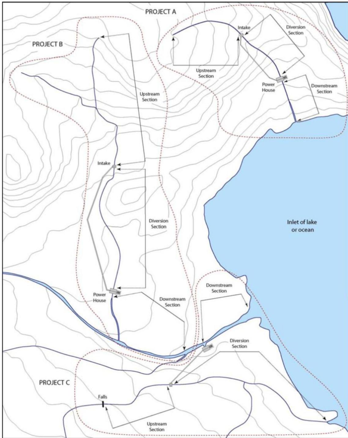
Figure 2. Examples of upstream, diversion, and downstream sections for three hypothetical hydroelectric projects (taken from Lewis et al. 2004).
